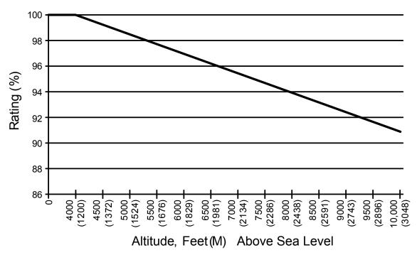
Operation at full load at a higher altitude can be accommodated in ambient temperatures less than 104°F (40°C) ambient. **Figure 2** shows the maximum allowable ambient temperature for full load operation at altitudes above 4000 feet (1200 m).
